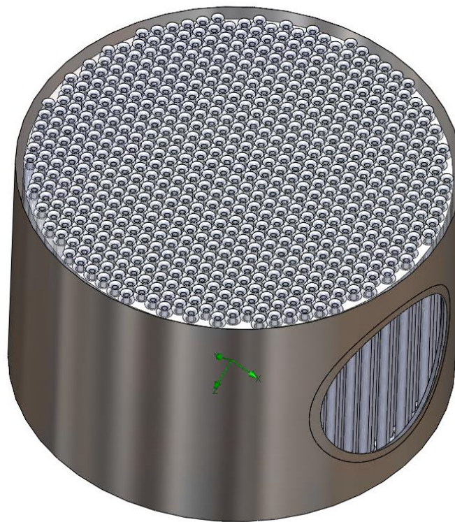
Figure 4-2: An overview of the optimized shell and tube geometry that is to be additively manufactured.
